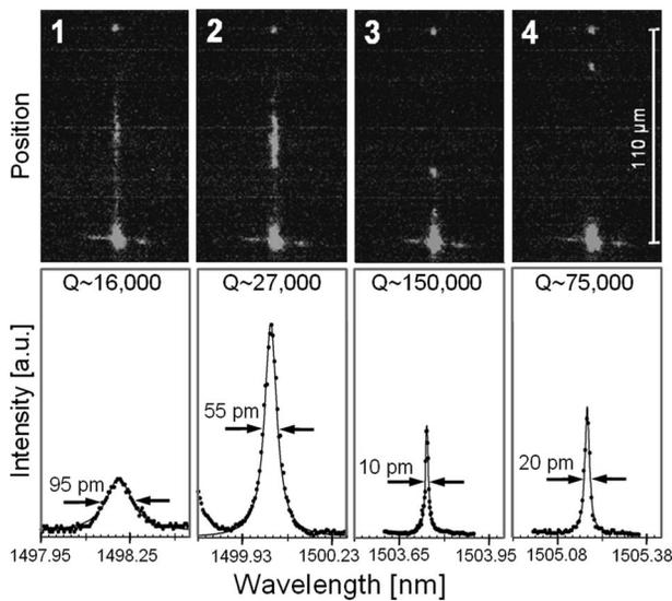
FIG. 4. Near infrared images of the scattered fields (top) and detailed spectra (bottom) for four wavelengths marked in Fig. 3. The light is incident from the bottom and the bright spot that marks the end of the waveguide and is present at all scanned wavelengths is caused by scattered light reflected to the waveguide's outlet from the other facet of the  $\sim 3$  mm long cleaved sample.
