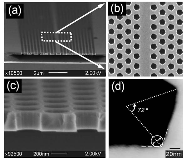
FIG. 2. (a) SEM image of the fabricated PhC slab, (b) top view of the randomized pattern, (c) detailed micrograph of the cleaved facet showing the tilt and the surface roughness of the etched wall, and (d) AFM image showing the top edge roughness and the rounded vertices of a pentagonal air hole.
