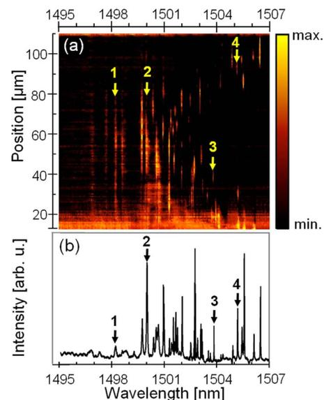
FIG. 3. (Color online) (a) Contour plot of spatially resolved spectra of the vertically dissipated light from a 110  $\mu\text{m}$  long disordered waveguide. Wavelength-scan step size is 5 pm. Spatial positions up to  $\sim 13$   $\mu\text{m}$  from the edge are not shown due to excessive surface scattering in that region. (b) Total, spatially integrated spectra of the same sample showing multiple Lorentzian-shaped resonances.
