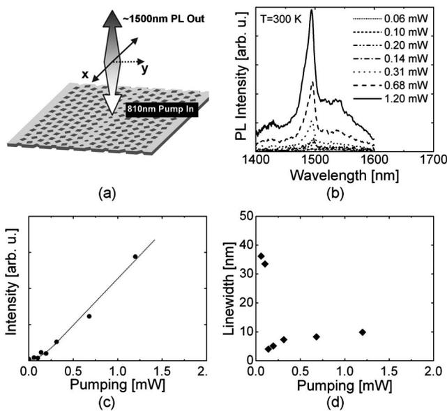
FIG. 3. (a) Schematic of the active cavity characterization scheme, (b) emission spectra of a silicon random PC microcavity with PbSe QDs measured at 300 K at different pump powers, (c)  $L$ - $L$  characteristics, and (d) emission peak linewidth vs pump powers.
