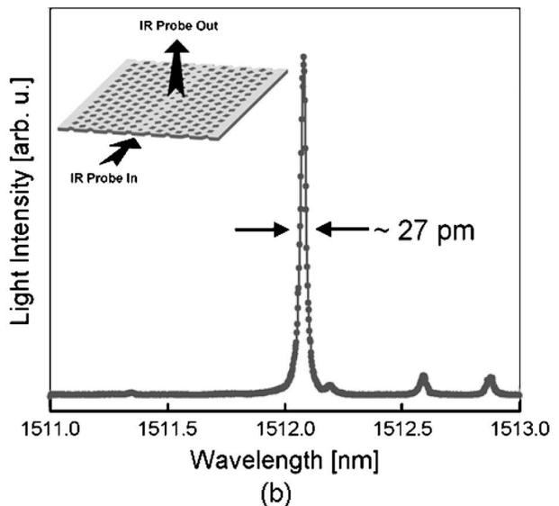
FIG. 2. (Color online) (a) Contour plot of the spatially resolved spectra of a  $150 \mu\text{m}$  long disordered waveguide. (b) Example of a well-localized, high- $Q$  resonance in the passive random PC microcavities. The probing and collection directions are indicated in the inset.
