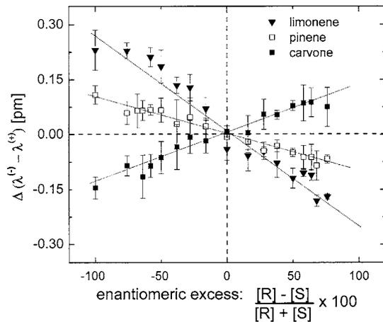
Fig. 3. Change in the spacing of left (-) and right (+) circularly polarized resonant modes as a function of the enantiomeric excess. [R] and [S], respectively, denote the concentrations of the liquids' R and S enantiomers. The lines are linear fits to the data.
