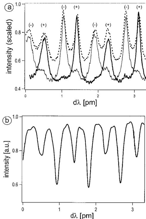
Fig. 2. (a) Transmission spectra (raw data) of limonone and a wavelength scan of  $\sim 763$  nm +  $d\lambda$  recorded by photodetector D2 (see Fig. 1). Spectra are shown after polarization analysis for either left (-) or right (+) circularly polarized modes (respectively, thin and thick solid curves) or for a scan without polarization analysis (dotted curve). For details see text. (b) Corresponding transmission spectrum (raw data) recorded with photodetector D1 (Fig. 1).
